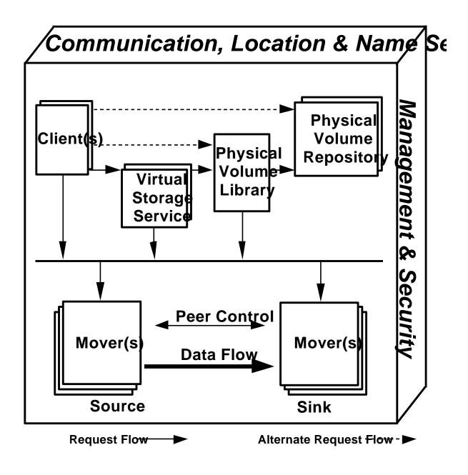
Figure 1. Reference Model for Open Storage Systems Interconnection
