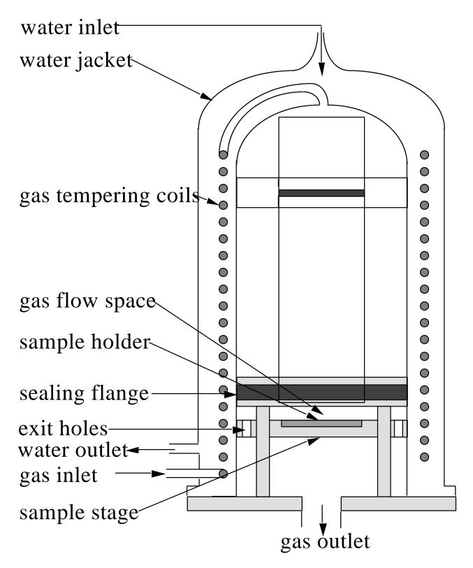
Figure 3. Detailed schematic of the impinging jet chamber
