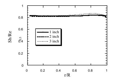
Figure 7. The uniformity of mass transfer to samples. Heights of the nozzles above the sample stage: 1 inch: 0.177"; 2 inch: 0.390"; 3 inch: 0.600". The heights should be within +/- 0.010" of the indicated values.
