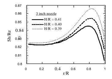
Figure 6. The dimensionless local mass transfer coefficient on the surface of impingement as a function of radius from the axis of the 3 inch nozzle. In the case of H/R = 0.40, the maximum nonuniformity is +/- 0.018 or about 2% of the average value.
