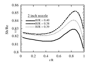
Figure 5. The dimensionless local mass transfer coefficient on the surface of impingement as a function of radius from the axis of the 2 inch nozzle. In the case of H/R = 0.39, the maximum nonuniformity is +/- 0.012 or about 1.5% of the average value.
