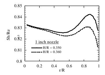
Figure 4. The dimensionless local mass transfer coefficient on the surface of impingement as a function of radius from the axis of the 1 inch nozzle. In the case of H/R = 0.35, the maximum nonuniformity is +/- 0.0085 or about 1% of the average value.
