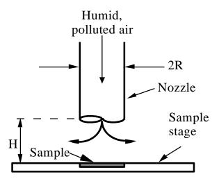
Figure 1. A schematic diagram of the impinging jet
