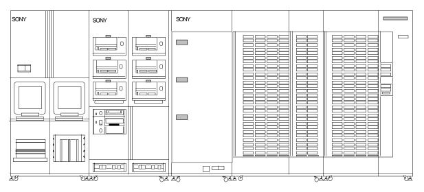
Figure 1. Master Data Storage Subsystem (MDSS)
