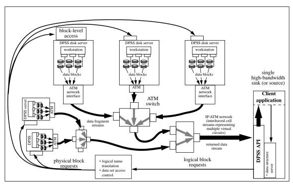
Figure 2 Distributed-Parallel Storage System Implementation
