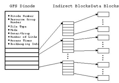
Figure 4: GFS Dinode Internal Structure
