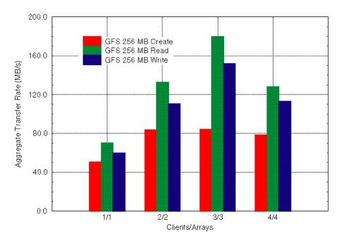
Figure 8: Aggregate Transfer Rate of 256 Mbyte Files.
