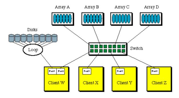
Figure 5: GFS Hardware Configuration for Tests Performed May 1997.
