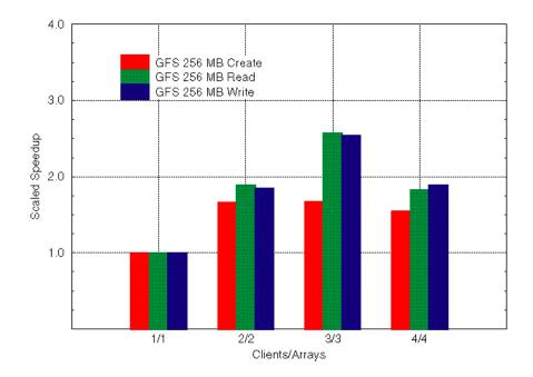
Figure 9: Scaled Speedup for 256 Mbyte File.
