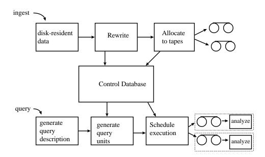
Figure 1: Data warehousing architecture.
