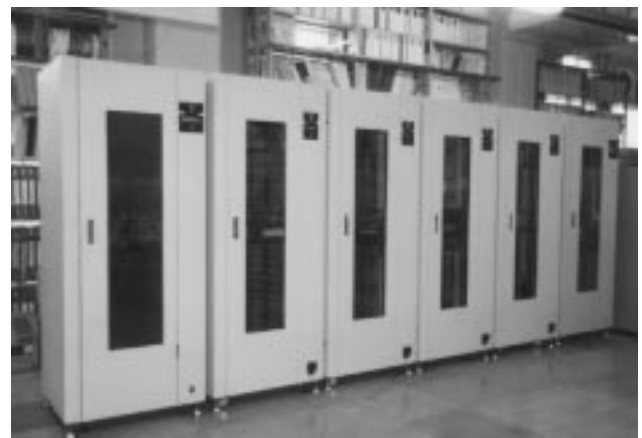
Figure 4. Photograph of scalable tape archiver
