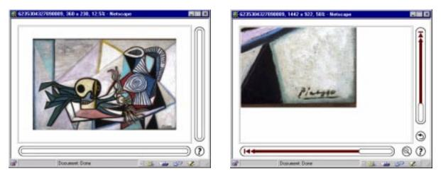
Figures 2(c) and 2(d): The GridPix viewer. Figure 2(c) shows a Picasso art work at 12.5% resolution within the GridPix viewer. Figure 2(d) shows the artist's signature at the lower right hand corner of the same image, at 50% resolution. Since the entire image appears in the viewer at 12.5% resolution, no scrollbars are displayed. Since JPEG is grid-based, tiles can be placed side by side in an HTML file and appear as if it is a single image.
