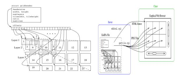
Figures 2(a) and 2(b): Figure 2(a) shows the structure of a GridPix file. Figure 2(b) shows how image tiles are displayed in a graphical browser created using HTML
