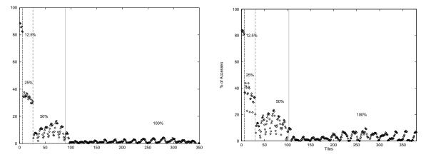
Figures 8(a) and 8(b): Frequency of tile access for the top two images. Tiles are numbered starting from the top left hand corner of the 12.5% resolution version. Vertical lines separate the tiles from each resolution
