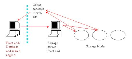
Figure 1: How the site works. Clients access images through a keyword search at the front end. Once an image is selected, tiles are transferred to the client from a storage server that is holding the image. The storage servers are managed by a storage front end. The vertical line separating the database and storage system indicates that these two servers are in different geographical locations.
