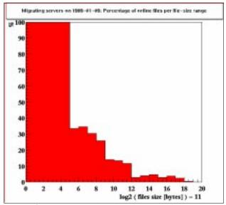
Figure 6: Percentage of on-line files per file-size range on wiping fileservers. All files < 64 KB are online because they are stored in the local disk partition.
