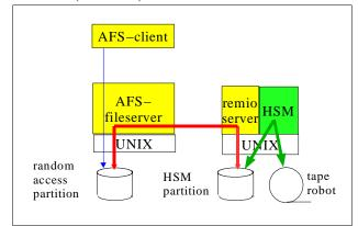
Figure 1: The AFS-client is served from a random access residency (blue arrow). The fileserver copies files to the HSM-partition (red arrow) where the HSMsystem writes them onto tape (green arrow).
