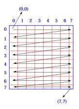
Figure 1: A global tape-resident array divided into 64 chunks.
