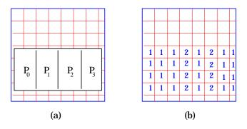
Figure 3: (a) An access pattern involving four processors. (b) The global array with each sub-file marked with the number of processors that share it.
