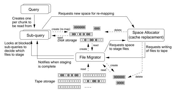
Figure 6: System components and their interactions
