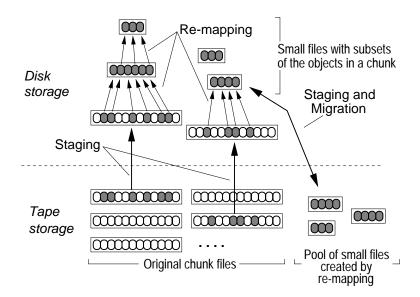
Figure 4: Overview of the complete storage architecture
