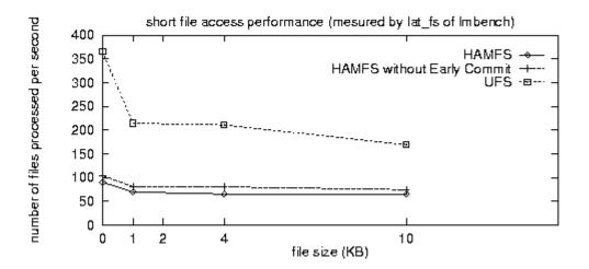
Figure 8: Short file access with high-speed disk array
