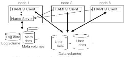
Figure 2: Configuration of HAMFS file system
