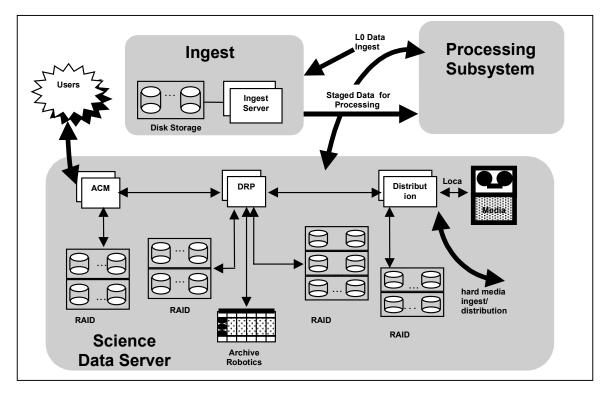
Figure 1. Hardware Configuration of the ECS Archive
