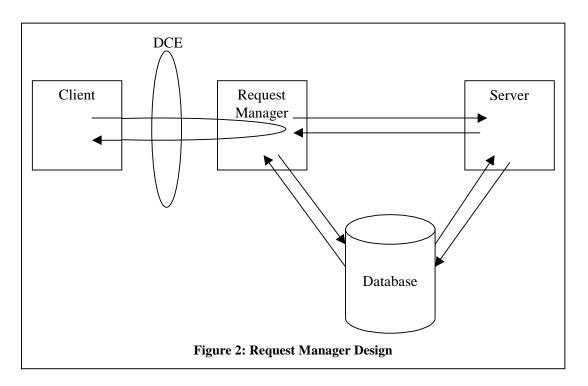
By using the database as the request queue, the Request Manager permits virtually unlimited requests to be queued. Moreover, priority-based dequeueing can be enforced
