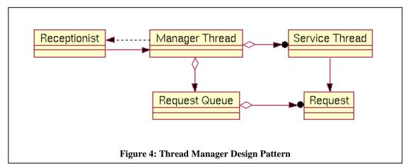
The manager thread controls the assignment of requests from the queue to the pool of service threads. It waits on a condition variable until such time as it is notified by the receptionist that new work has arrived in the queue, or by a service thread that the service thread has completed its work and is ready for a new assignment. Restrictions are placed neither on the number of requests in the queue, nor on the number of service threads available for assignment.
