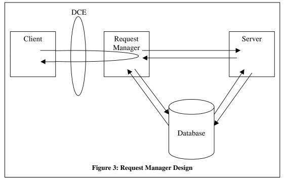
via the SQL stored procedures that are used to select the next available request for servicing. Stored procedures are also used to implement the routing logic, permitting adjustments to routing to be made strictly through database patches.
