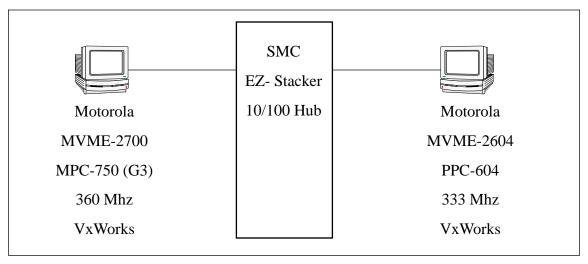
Figure 8. Hardware Configuration
