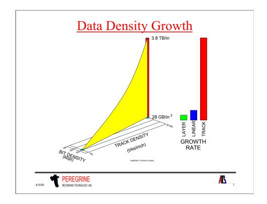
As can be seen from figure. 7, most of this increase comes from increasing track density. The current limits to the track density are:
