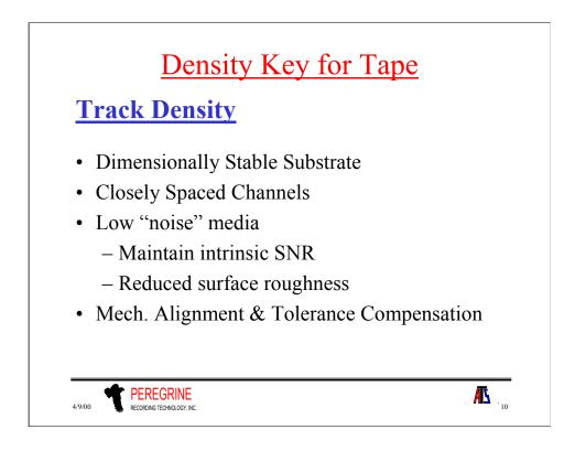
The NSIC program projects a 25X increase in track density. The keys to achieving this are to find a dimensionally stable substrate across the environmental extremes the cartridge is likely to experience and to reduce the multi-channel element span by placing the elements closer together.
