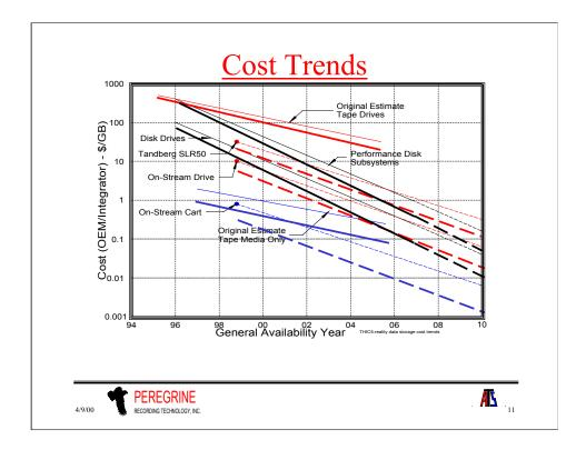
The current evolutionary path for tape does show that the cost/bit for a disk drive will soon fall below that of tape. With the aggressive volumetric density increase proposed here, this will not happen. Tape capacity and, hence, cost/bit will keep up with disk drives.
