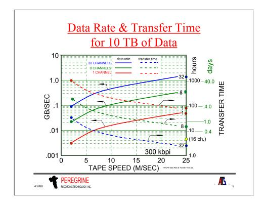
A significant problem for both disk and tape is how to transfer all the data in a reasonable time. Suppose for a moment that a cartridge is filled with 10 TB of data. Even at a high tape speed of 25 meters/sec, multiple channels are required. A single channel device, operating at 100 percent efficiency would take nearly **four days** to transfer the data.
