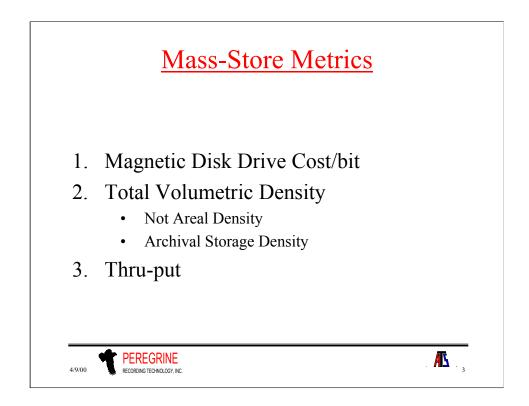
The common metric for all storage is the cost/bit of disk drives which continues to fall at a rate of almost 50 percent per year. Any mass storage technology must be at a fraction of the cost of disk drive storage at the time of its introduction.
