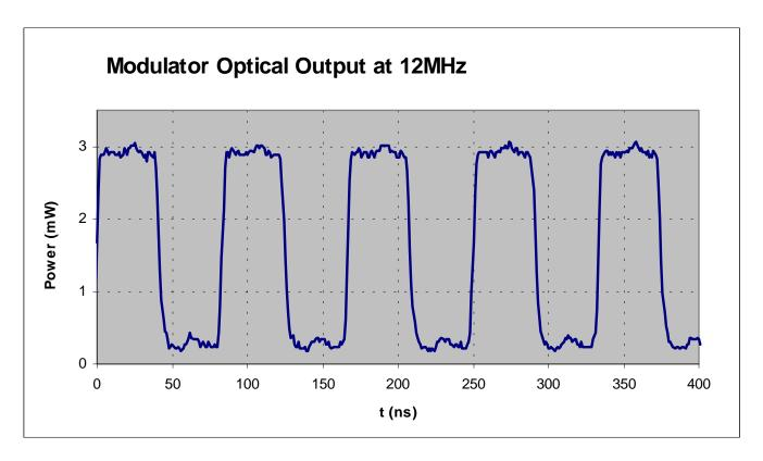
Optical Modulation @ 12MHz provides PPM data at 16.7 Mbits/sec. per track, e.g. 64 tracks = 1069 Mbits/sec. ⇒ 800 Mbit/sec. User Data Rate (34% O.H.)
