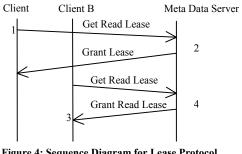
Figure 4: Sequence Diagram for Lease Protocol Interactions (Read-Sharing Case)
