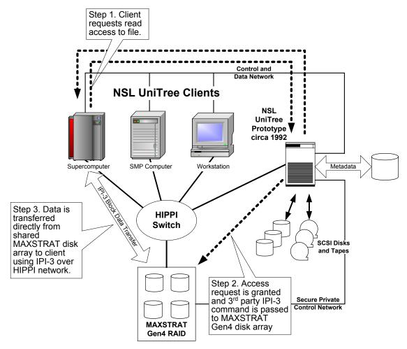
Figure 3: The NSL Prototype provided 3<sup>rd</sup> party "LAN-less" data transfers.
