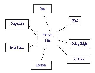
Figure 2. Star model diagram for ISH.
