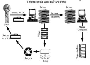
Figure 2. Recent interactive WSR-88D level II 8mm tape processing required nine workstations and 92 8mm tape drives
