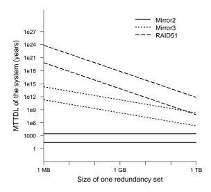
Figure 8. Mean time to data loss in a 2 PB storage system. The upper line for each configuration is for a system built from disks with a  $10^6$  hour MTTF, and the lower line for each configuration is for a system built from disks with a  $10^5$  hour MTTF.
