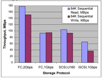
Plot 1. Streaming Read/Write performance measured by the lometer benchmark
