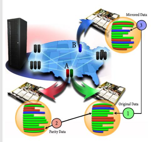
In this example a primary data image (1) is being protected with one dimension of local parity (2) and one dimension of global mirroring (3).
