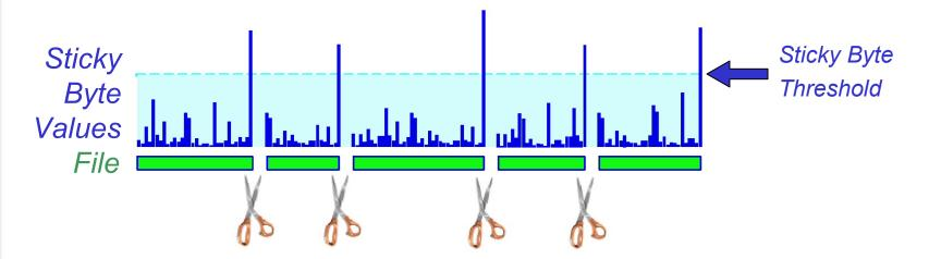
Sticky Byte Factoring orchestrates commonality by cutting large files into variable length chunks in a deterministic way.
