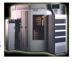
1987 6000 Slots @ 200 MB Max 16 Transports at 3MB/Sec Shared across 4 110 Exchanges/Hour Total Capacity – 1.2 TB Uncompressed 2002 6000 Slots @ 200 GB Max 80 Transports at 30MB/Sec Per Transport 450 Exchanges/Hour Total Capacity – 1.2 PB Uncompressed
