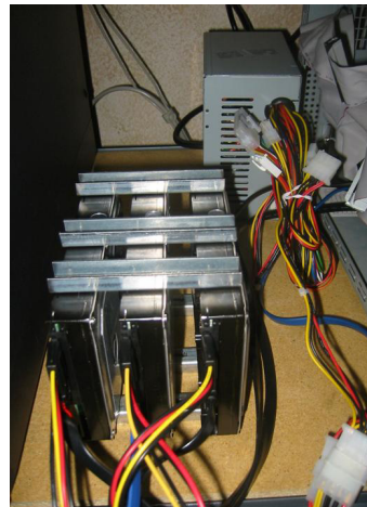
Figure 2. A stack of five 2.5-inch disk drives physically coupled with stiff metal rails.
