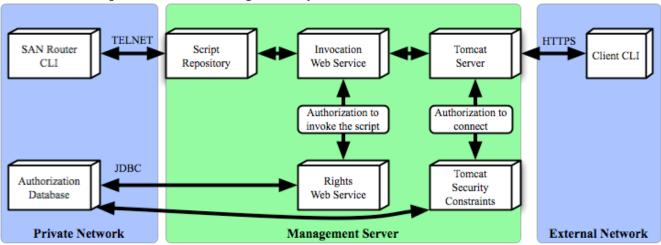
Figure 2. Software Components of the Management System
