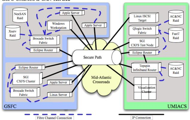
Figure 1. The GSFC-UMIACS IP SAN Testbed
