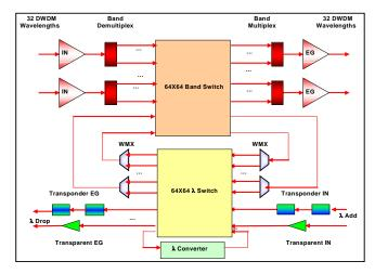
Figure 2. LambdaNode 2000 hardware architecture
