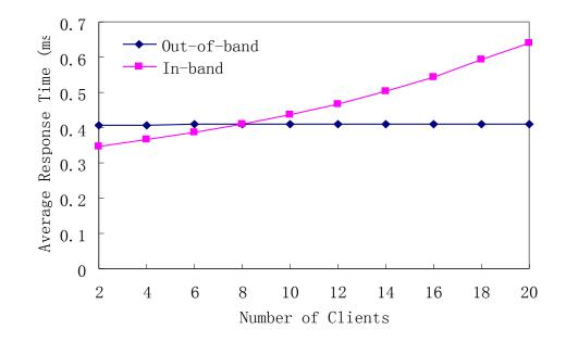
Average Response Time using ACQ of out-of-band compared with FBR of in-band less when host number > 10 increase much slower
