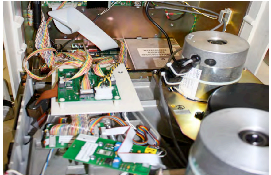
Custom bias and amplifiers tuned for weak bits
