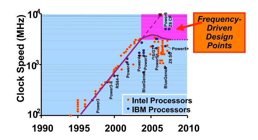
Power constrains benefits of frequency increases Consequence is the switch to multi-core systems
