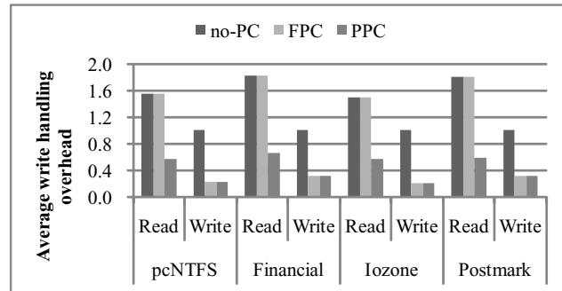
Fig. 7. Average write handling overheads (4+1 RAID-5)
