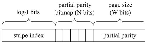
Fig. 2. The Entry of Partial Parity Cache
