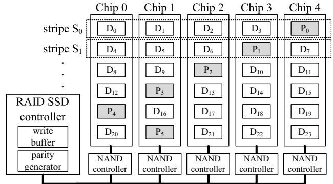
Fig. 1. 4+1 RAID-5 SSD Architecture
