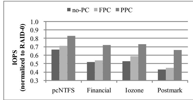
Fig. 6. I/O performances of no-PC, FPC and PPC schemes normalized by RAID-0 scheme (4+1 RAID-5)
