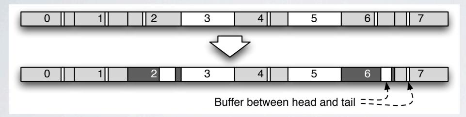
In-band compaction with circular logs
