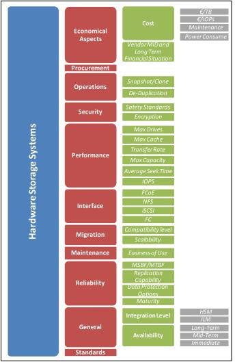
Figure 3. Evaluation Model for Hardware Storage Systems.
