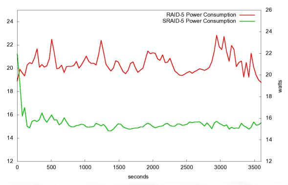
The S-RAID 5 includes 5 Seagate ST3500418AS 500G 7200RPM Disks, and is divided into 2 groups of 2 disks. The number of vertical group is set to 5, the same as the number of the disks.
