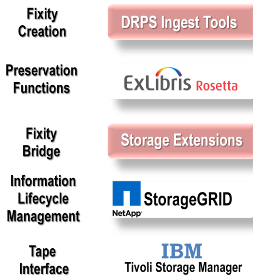
Architecture of the Church History Department's Digital Records Preservation System (DRPS)
