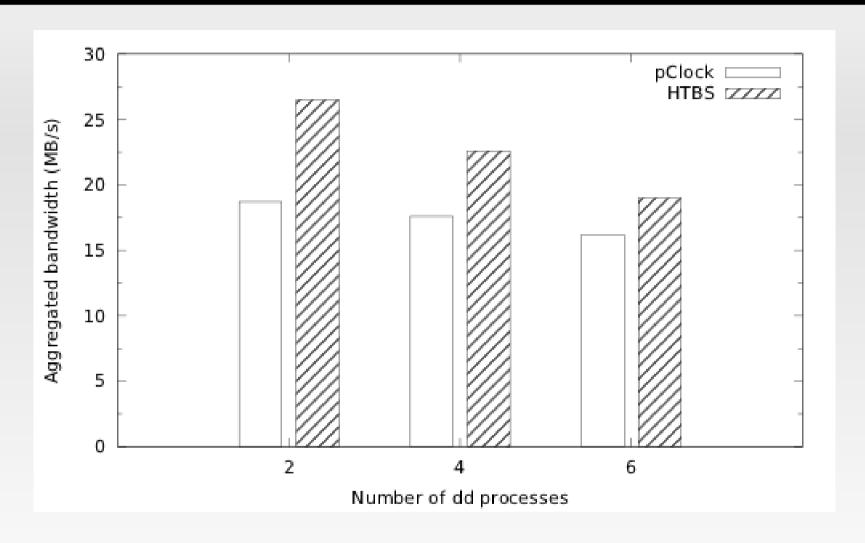
Aggregated bandwidth achieved by pClock and HTBS using *dd* processes
