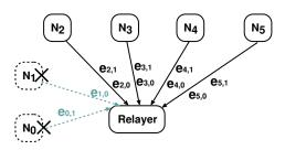
Fig. 3. An example of how the relayer downloads real and virtual symbols for a (6,3) code when there are two failed nodes  $N_0$  and  $N_1$ . Here,  $e_{1,0}$  and  $e_{0,1}$  are the virtual symbols.
