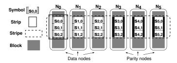
Fig. 1. Example of a distributed storage system, where n=6, k=3, and r=3. We assume that nodes  $N_0$ ,  $N_1$ , and  $N_2$  are data nodes, while  $N_3$ ,  $N_4$ , and  $N_5$  are parity nodes. For load balancing, the identities of data and parities nodes are rotated across different blocks.
