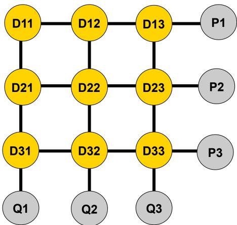
Tolerates all double disk failures
