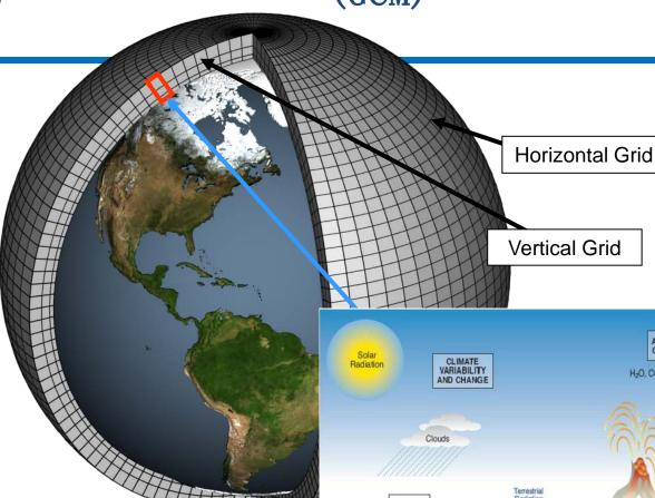
A GCM is a mathematical representation of the major climate system components and their interactions. The GCM equations operate on a global grid and are solved on a computer.
