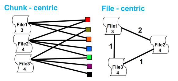
A simple on-tape chunk placement algorithm – that reduces seek time overhead due to chunk fragmentation.
