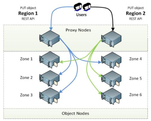
Proxy Nodes tie together the rest of the Swift architecture. For each request, it looks up the location of the account, container, or object and routes the request accordingly. The public REST API is exposed through the Proxy Nodes.
