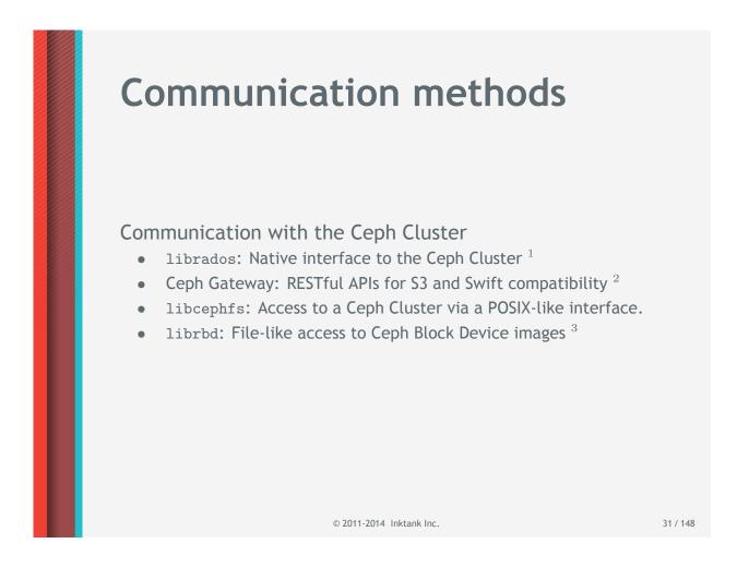
Note 1: Services interfaces built on top of this native interface include the Ceph Block Device, The Ceph Gateway, and the Ceph File System.
