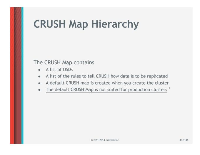
Note 1: This default CRUSH Map is fine for a sandbox-type installation only! For production clusters, it should be customized for better management, performance, and data security
