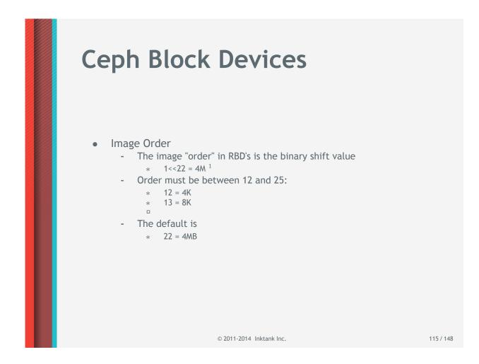
Note 1 : The << C operator is a left bit shifting operator. << shifts the left operand bits by the right operand value A binary value for example
