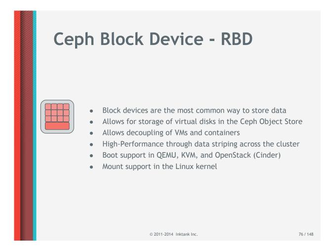
RBD stands for <u>RADOS</u> <u>Block</u> <u>Device</u> Date is striped across the Ceph cluster
