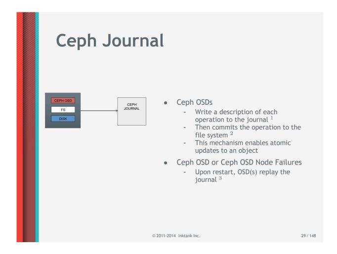
Note 1 : The write to the CEPH cluster will be acknowledged when the minimum number of replica journals have been written to.
