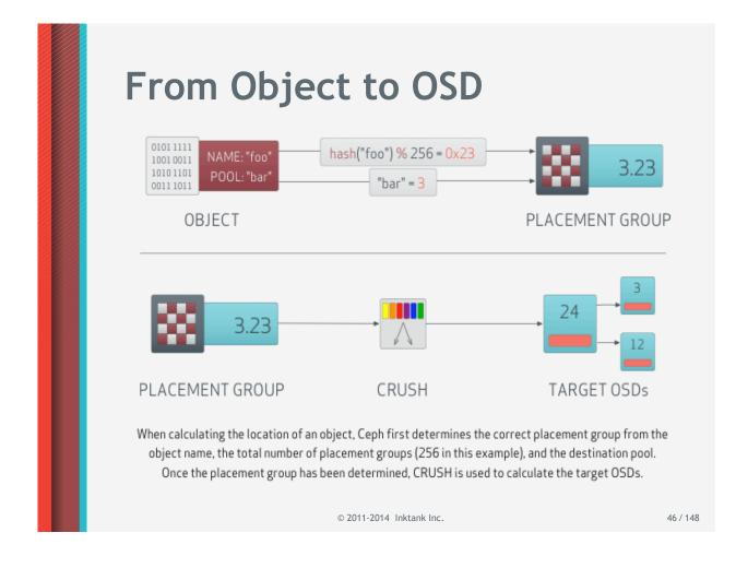
To generate the PG id, we use - The pool id - A hashing formula based on the object name modulo the number of PGs
