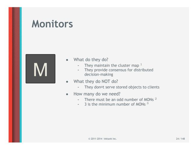
Note 1: Ceph Monitors are daemons. The primary role of a monitor is to maintain the state of the cluster by managing critical Ceph Cluster state and configuration information. The Ceph Monitors maintain a master copy of the CRUSH Map and Ceph Daemons and Clients can check in periodically with the monitors to be sure they have the most recent copy of the map.
