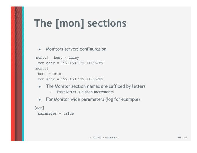
Ceph-deploy build by default a default ceph.conf file
