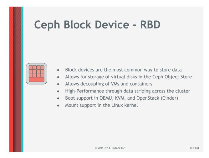
RBD stands for <u>RADOS</u> <u>Block</u> <u>Device</u> Date is striped across the Ceph cluster
