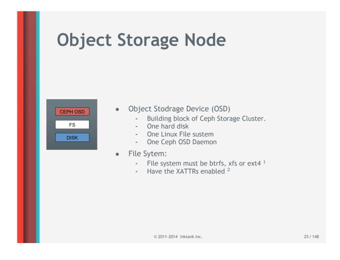
The OSD connect a disk to the Ceph Storage Cluster
