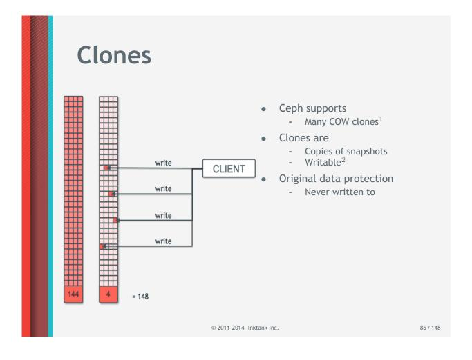
Note 1 : Reads are always served from the original snapshot used to create the clone. Ceph supports many copy-on-write clones of a snapshot
