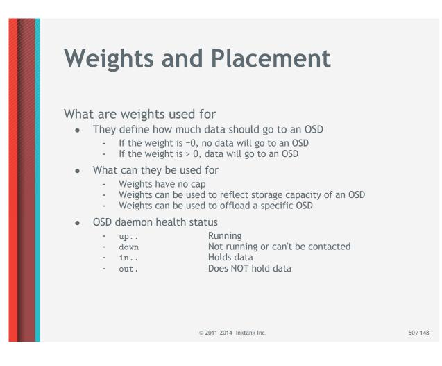
As a quick way to remember it, the weight value indicates the proportion of data an OSD will hold if it is up and running
