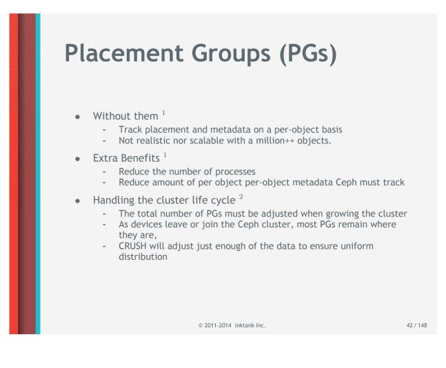
Note 1: Tracking object placement and object metadata on a per-object basis is computationally expensive-i.e., a system with millions of objects cannot realistically track placement on a per-object basis. Placement groups address this barrier to performance and scalability. Additionally, placement groups reduce the number of processes and the amount of per-object metadata Ceph must track when storing and retrieving data.
