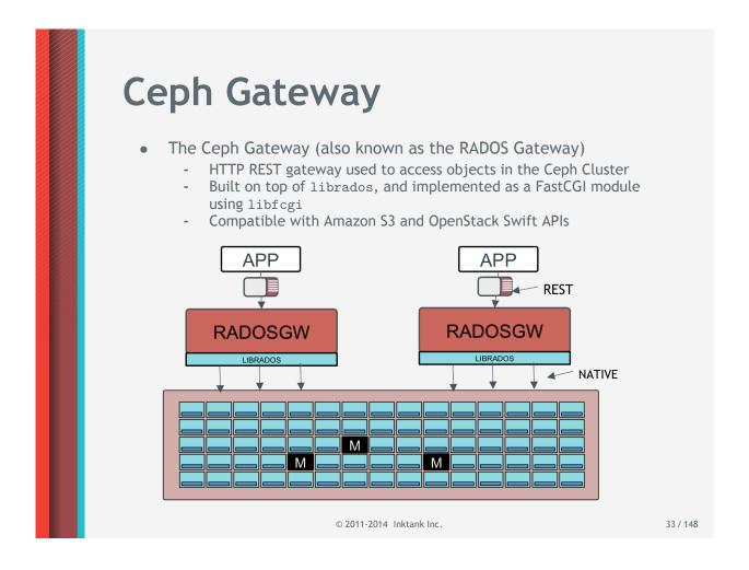
The gateway application sits on top of a webserver, it uses the librados library to communicate with the CEPH cluster and will write to OSD processes directly.
