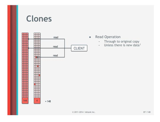
Note 1 : If data has been updated in the clone, data is read from the clone mounted on the host.
