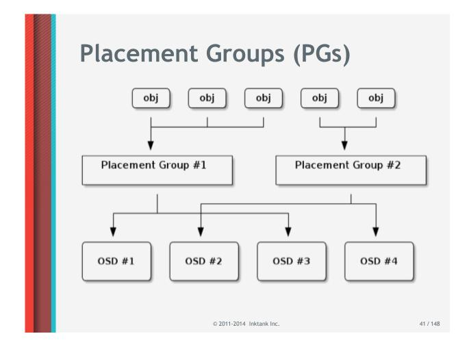
A Placement Group (PG) aggregates a series of objects onto a group, and maps the group to a series of OSDs.
