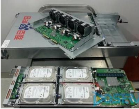
Fig. 1: Photo of Baidu’s ARM-based servers.
