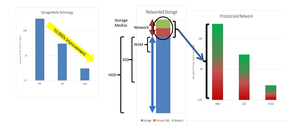
Faster Networking, Protocol Offloads, & Bypass Required to Match NVM Performance
