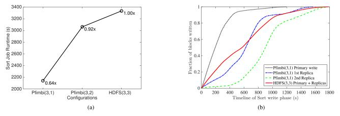
Fig. 9: Sort job under HDFS and Pfimbi. (a) Pfimbi improves Sort runtime. (b) The primary writes (black) and first replicas (blue) complete faster in Pfimbi. The second replicas (green) complete on par with HDFS(3,3).
