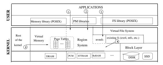
Fig. 2. A PM-specific memory/storage stack – ① Applications use PM directly using region system interfaces. ② Applications consume PM through PM libraries (e.g. pmem.io), which can use region system or PM-specific file systems to access PM. ③ Applications access PM using traditional POSIX interface through ④ Applications using PM using traditional file systems. ⑤ Rest of the kernel accessing PM using region system.
