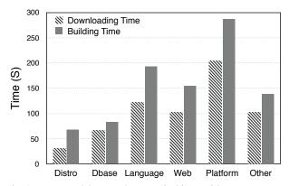
Fig. 3. Comparison of the times for image building and for retrieving remote input files. Each time is an average over all the times for different Dockerfiles versions of different base images in a base image group
