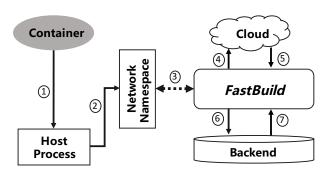
Fig. 4. Steps for FastBuild to redirect requests for input files and to access the cache
