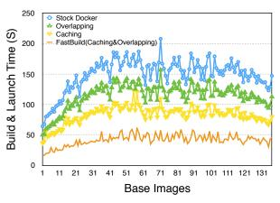
Fig. 6. The build and launch time for each sequence of Dockerfiles associated with a base image. The times for each of the 137 base images are shown for the stock Docker, FastBuild with only overlaping technique, FastBuild with only caching technique, and FastBuild with both techniques. The base images are shown in the order as they appear in Table I
