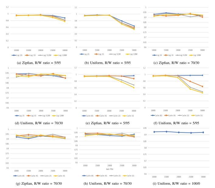
Fig. 7: Normalized total throughput of four instances. Numbers of X-axis stand for inserted records to each database, and numbers of Y-axis stand for normalized throughput. (a) to (d): Fix 4GB cache size and adjust log buffer size from 2GB to 128MB. (e) to (h): Fix the 2GB log buffer and change cache size from 8GB to 1GB. (i) 100% read uniform request.
