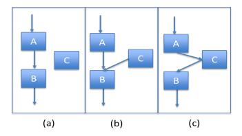
Fig. 5: The correct order of pointer updates for the objects of linked lists in NVM. From (a) to (c) is for the object insertion; from (c) to (a) is for object deletion.
