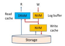
Fig. 1: The read/write data flow of vNVML private mmapping between DRAM, NVM, and storage device.
