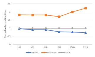
(b) Normalized vNVML and SoftWrap execution time assuming unlimited NVM size.
