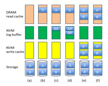
Fig. 2: The flow of read/write data of vNVML.
