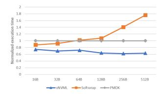
(a) Normalized vNVML and SoftWrap execution time with the same NVM size.
